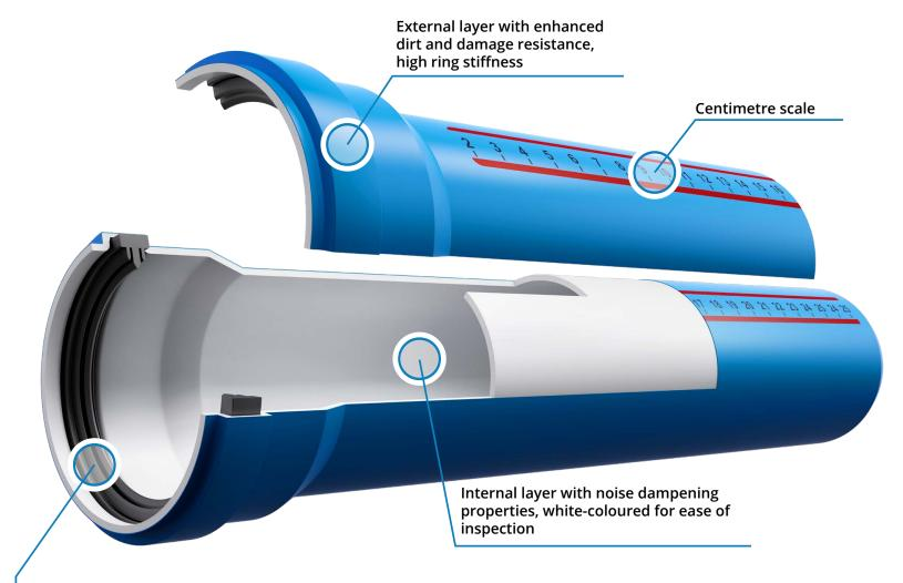
Triple lip seal (applies to Ø110 & Ø125 & Ø160) improves noise absorption and reliability of connections, ensures pressure resistance up to 4.5 bar
